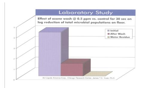
The graph above shows the effectiveness of ozone in the surface sanitation at a concentration of 0.5ppm. Taken from laboratory analysis of the DEL Ozone AGW-0500 by Air Liquide America Corporation. (Graphic courtesy of DEL Ozone.)
